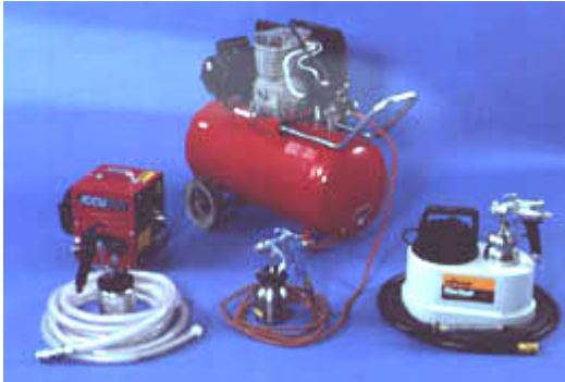
Here are samples of three different types of HVLP sprayers. The three-stage turbine-based Accuspray 23i, left, the Binks Mach I CAS gun in the middle, and the single-stage Wagner Professional FineCoat.
